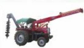
POST HOLE DIGGER & CRANE T-1
